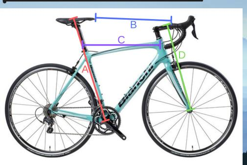
A. Center of bottom bracket to top of the saddle
